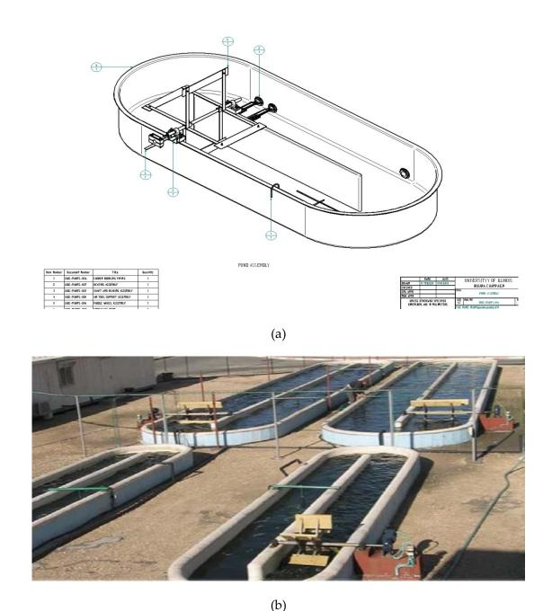
**Figure 1.** (a) Isometric drawing of algae pond constructed by UIUC students for study abroad program in South Africa (b) Picture of algae ponds operated by SeamBiotic in Ashkalon, Israel.
