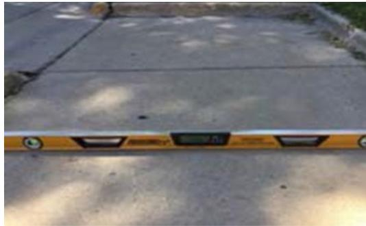
Figure 14 – Curb Ramp Cross Slope
